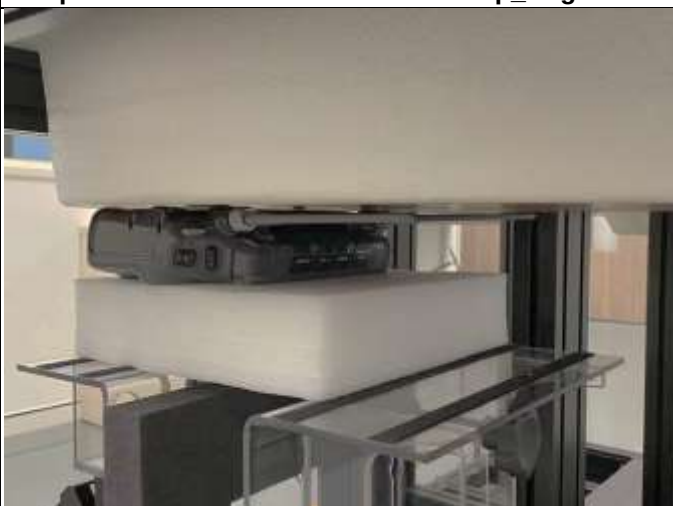
Inside of SDR-antenna 1 with 0.5cm Gap_Degree180
