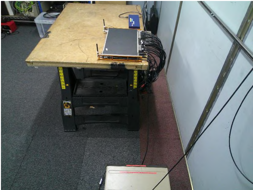
EUT powered using a 120VAC 60Hz power source
