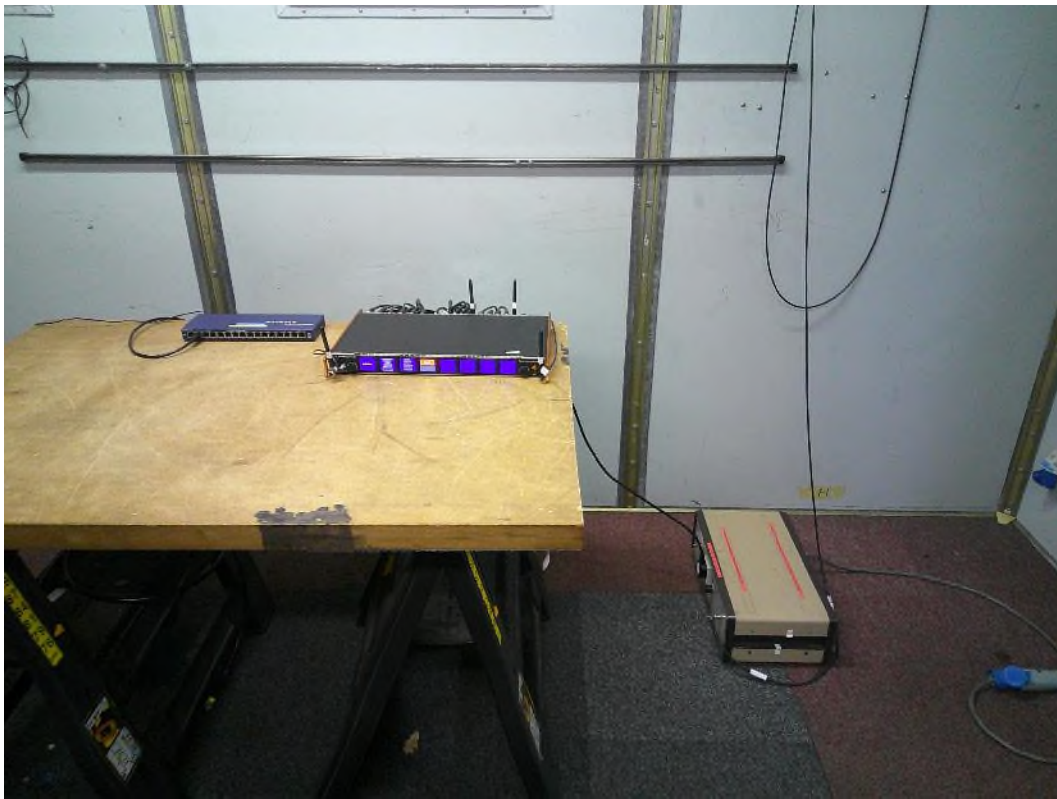
EUT powered using a 120VAC 60Hz power source
