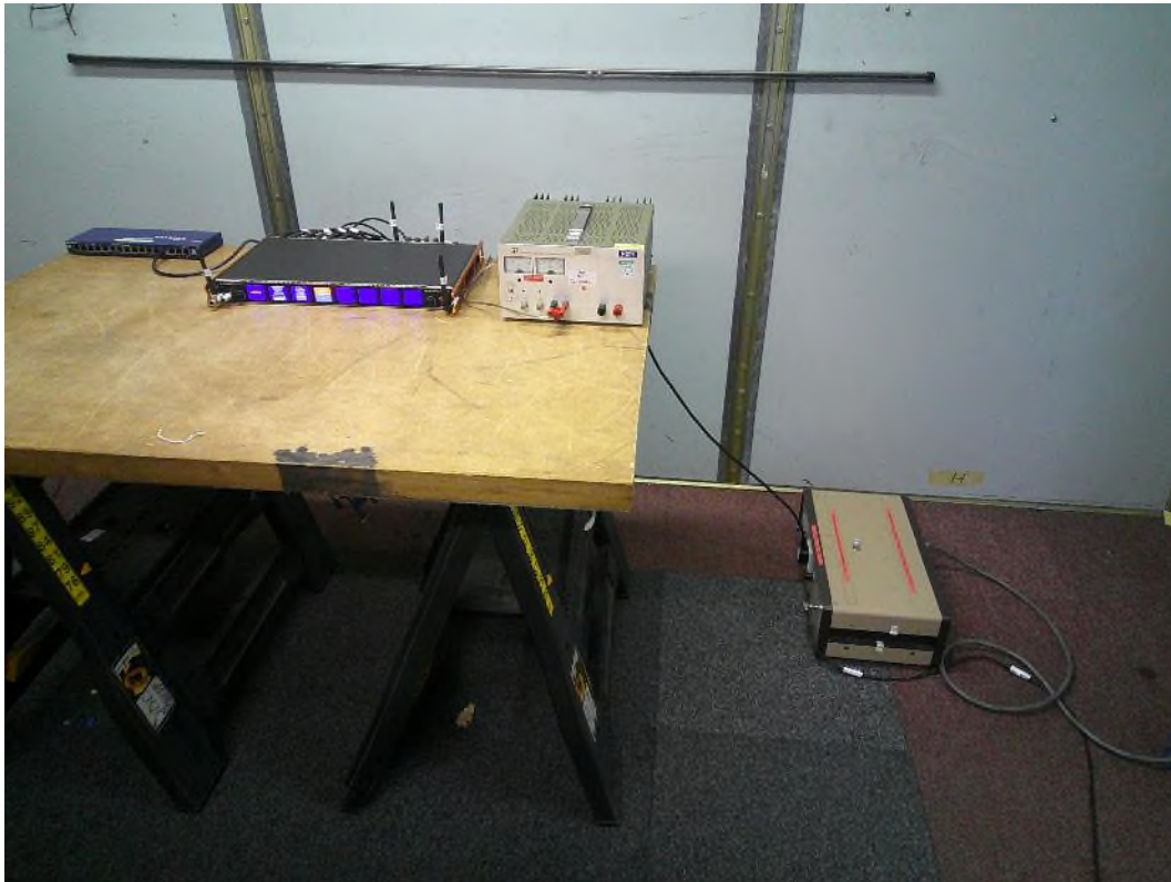
EUT powered via DC port using a bench power supply
