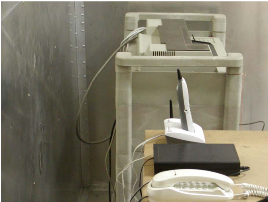
Conducted Emission - Side View (Model: GH3110 & GH3100)
