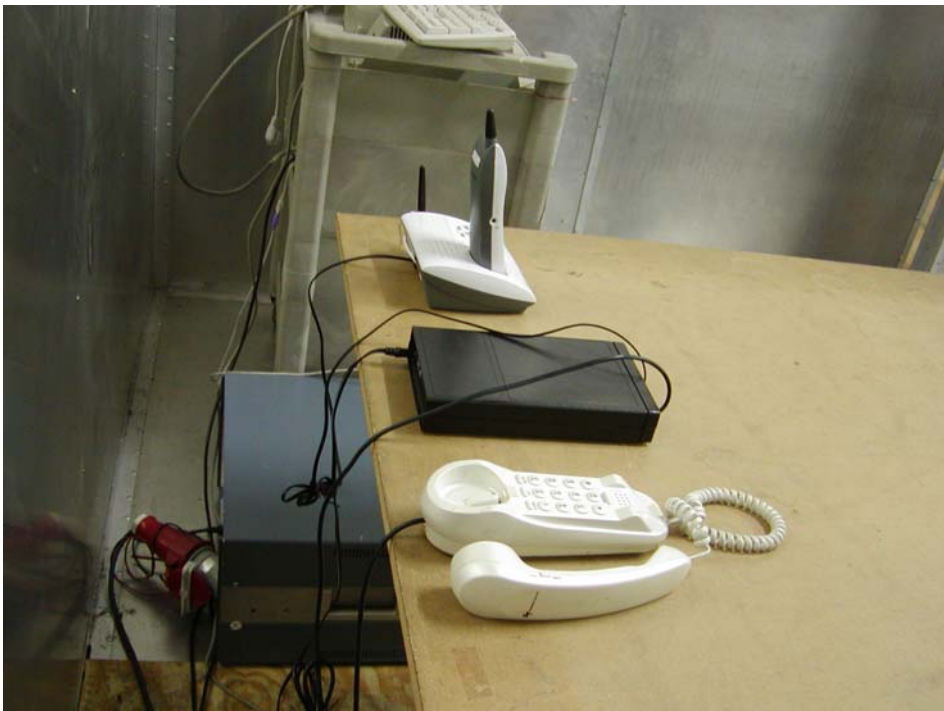
Conducted Emission - Side View (Model: GH3150)
