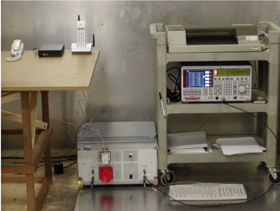
Conducted Emission - Front View (Model: GH3110 & GH3100)
