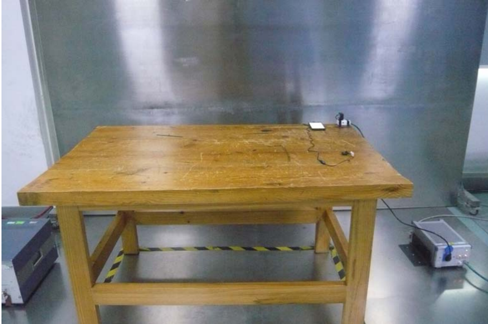
Conducted Emissions – Front View
