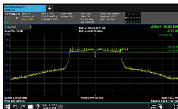
Figure 174 - 802.11n HT40 Maximum 6 dB EBW
