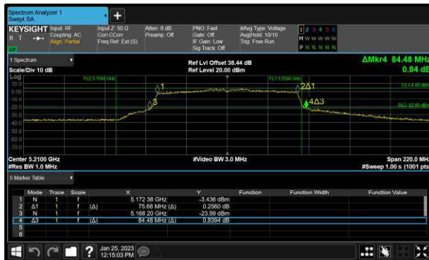
Figure 217 - 802.11ac VHT80 Minimum 99% OBW
