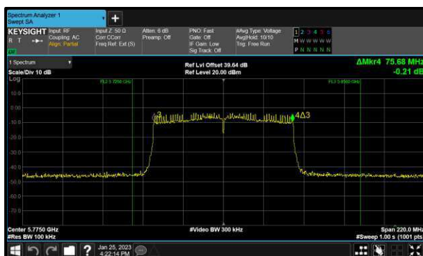
Figure 205 - 802.11ac VHT80 Minimum 6 dB EBW
