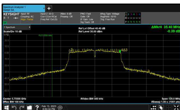
Figure 173 - 802.11n HT40 Minimum 6 dB EBW
