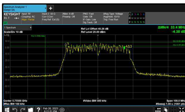
Figure 259 - 802.11ac HT40 Minimum 6 dB EBW
