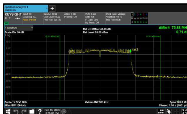
Figure 176 - 802.11ac VHT80 Maximum 6 dB EBW
