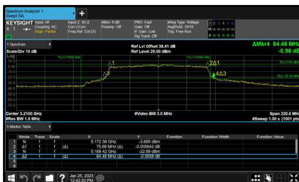
Figure 245 - 802.11ac VHT80 Minimum 99% OBW
