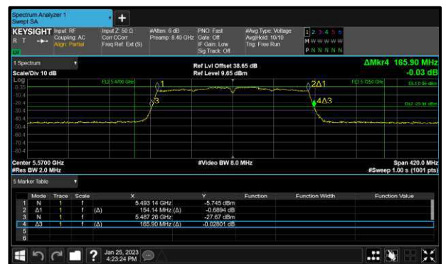
Figure 220 - 802.11ac VHT160 Maximum 99% OBW
