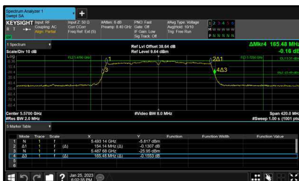
Figure 247 - 802.11ac VHT160 Minimum 99% OBW
