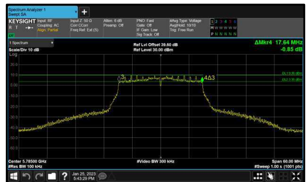
Figure 230 - 802.11n HT20 Maximum 6 dB EBW
