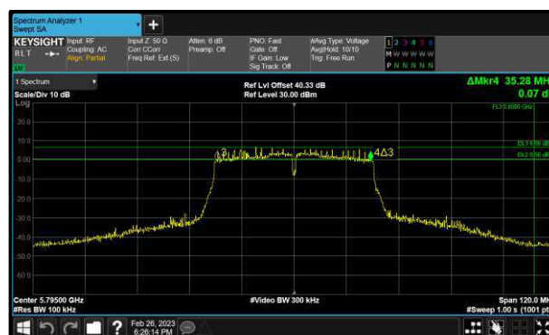
Figure 258 - 802.11ac HT20 Maximum 6 dB EBW
