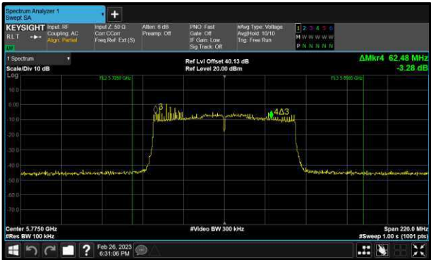
Figure 262 - 802.11ac VHT80 Maximum 6 dB EBW
