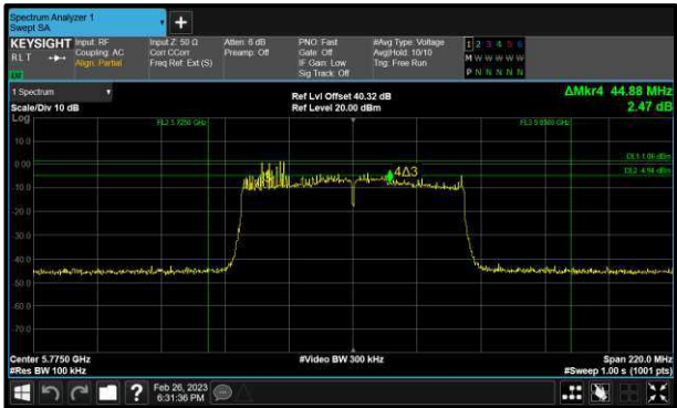
Figure 261 - 802.11ac VHT80 Minimum 6 dB EBW
