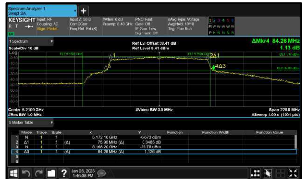
Figure 218 - 802.11ac VHT80 Maximum 99% OBW
