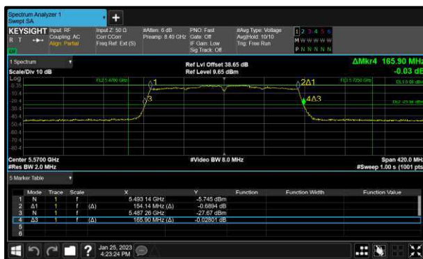
Figure 219 - 802.11ac VHT160 Minimum 99% OBW
