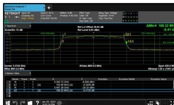
Figure 248 - 802.11ac VHT160 Maximum 99% OBW
