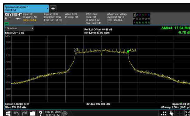
Figure 172 - 802.11n HT20 Maximum 6 dB EBW
