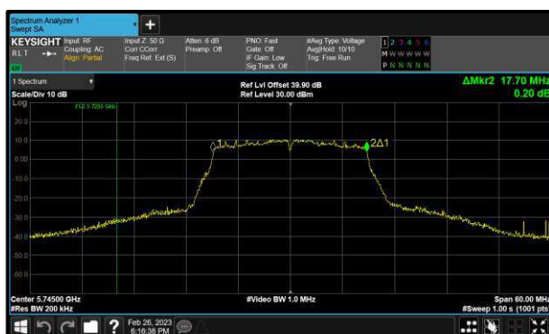
Figure 257 - 802.11ac HT20 Minimum 6 dB EBW
