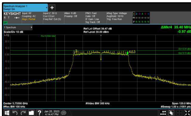
Figure 203 - 802.11n HT40 Minimum 6 dB EBW
