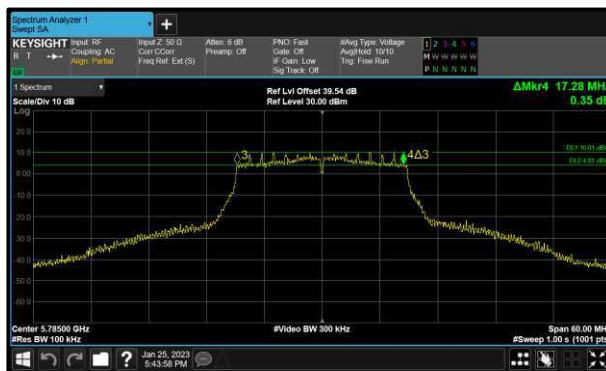
Figure 229 - 802.11n HT20 Minimum 6 dB EBW
