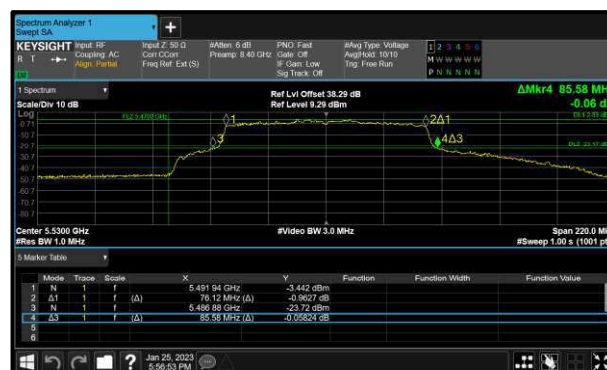
Figure 246 - 802.11ac VHT80 Maximum 99% OBW
