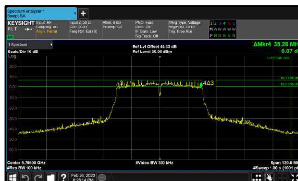
Figure 260 - 802.11ac HT40 Maximum 6 dB EBW
