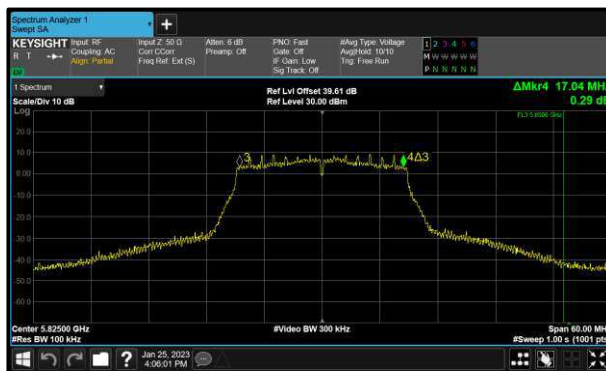
Figure 201 - 802.11n HT20 Minimum 6 dB EBW
