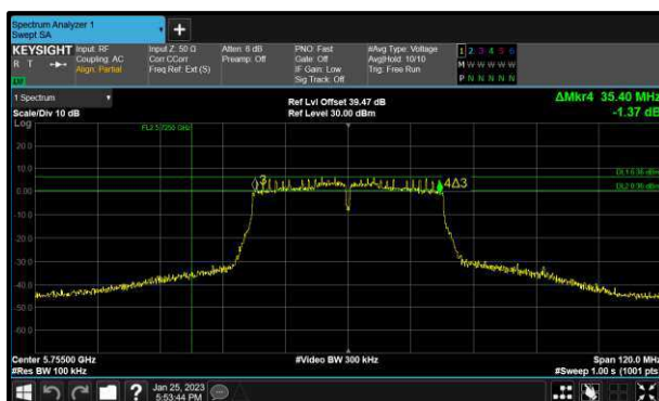
Figure 231 - 802.11n HT40 Minimum 6 dB EBW
