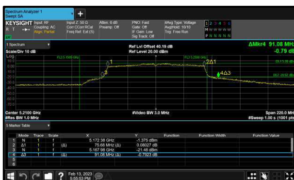
Figure 189 - 802.11ac VHT80 Minimum 99% OBW
