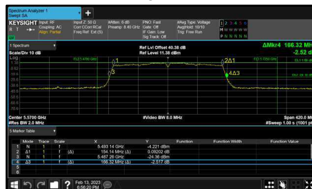
Figure 192 - 802.11ac VHT160 Maximum 99% OBW
