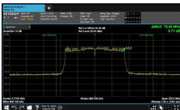
Figure 175 - 802.11ac VHT80 Minimum 6 dB EBW
