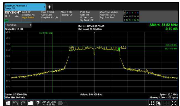
Figure 204 - 802.11n HT40 Maximum 6 dB EBW
