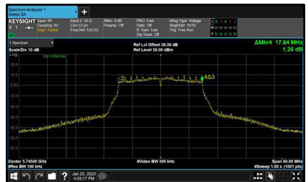
Figure 202 - 802.11n HT20 Maximum 6 dB EBW
