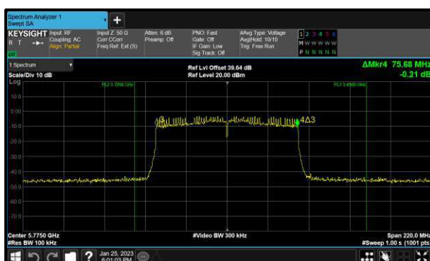
Figure 233 - 802.11ac VHT80 Minimum 6 dB EBW
