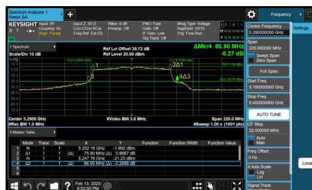
Figure 190 - 802.11ac VHT80 Maximum 99% OBW
