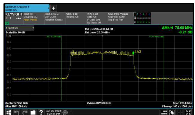
Figure 206 - 802.11ac VHT80 Maximum 6 dB EBW
