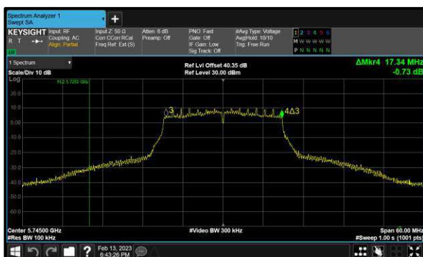
Figure 171 - 802.11n HT20 Minimum 6 dB EBW
