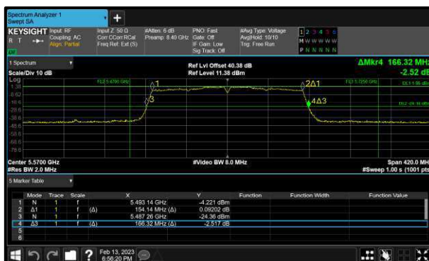
Figure 191 - 802.11ac VHT160 Minimum 99% OBW
