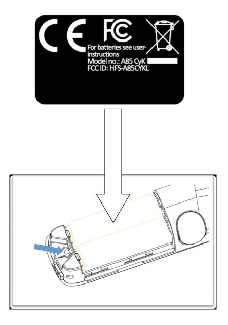
The Label stick inside the battery tank recess, which must be seen when remove the battery cover before using it.
