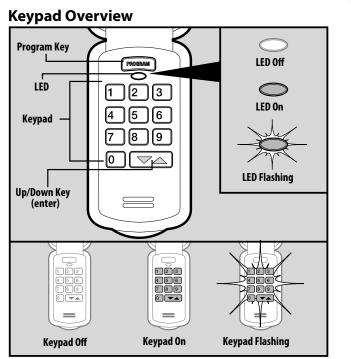
Activate keypad by opening battery compartment and pull protective tab. Reinstall compartment door to begin programming.
