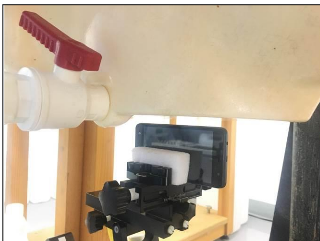
Left Side of EUT with 1.0 cm Gap
