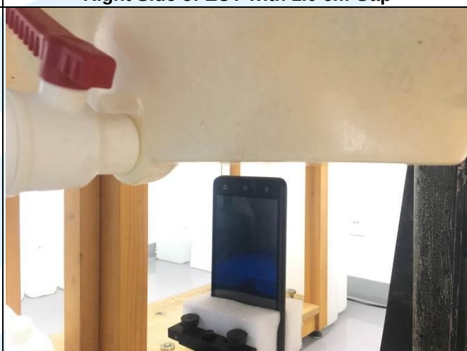
Bottom Side of EUT with 1.0 cm Gap
