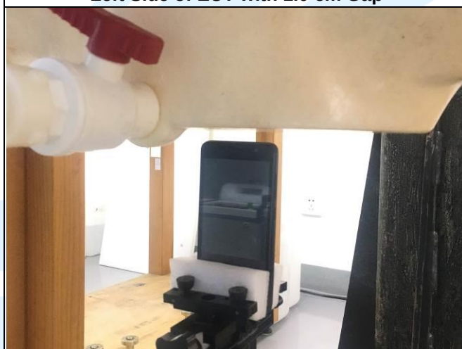
Top Side of EUT with 1.0 cm Gap
