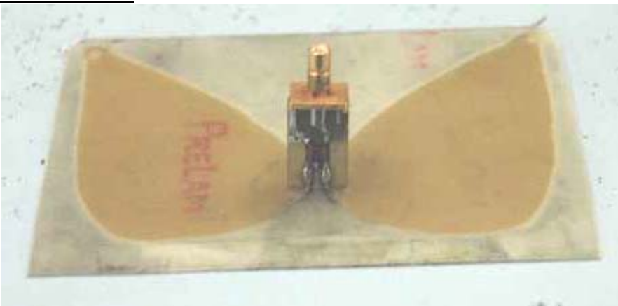
Balun PCA shown attached to Fan. Shrink wrap removed from Balun.
