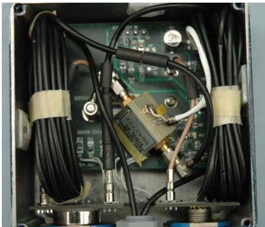
Electronics box shown with bagged shielding removed
