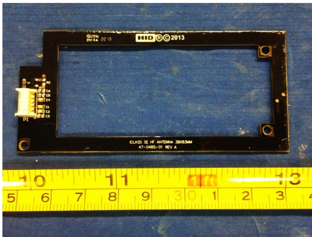
High Frequency Long Antenna Top View
