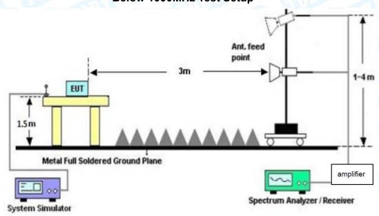
**Above 1GHz Test Setup**
