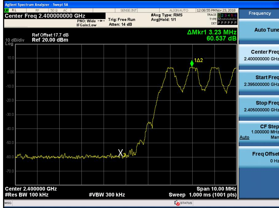
Test Plots with hopping (GFSK)
