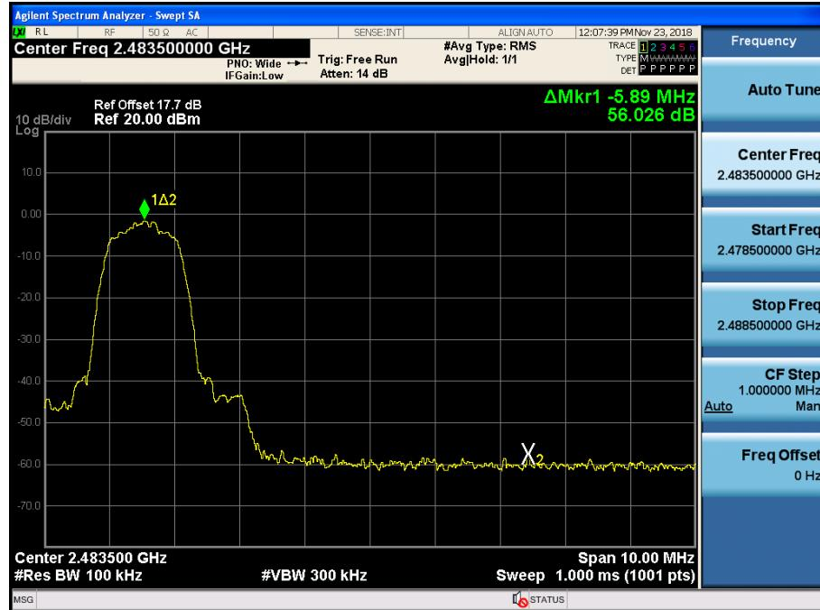
Test Plots with hopping (GFSK)
