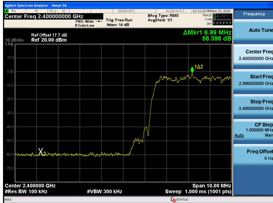
Test Plots with hopping (8DPSK)
