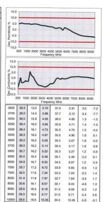
Figure D-2 600 - 10000 MHz Head Tissue Equivalent Matter
