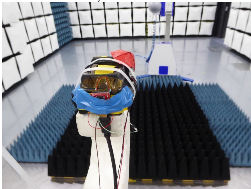
EUT on positioner Test setup fully anechoic chamber M276 Preliminary and final measurement
