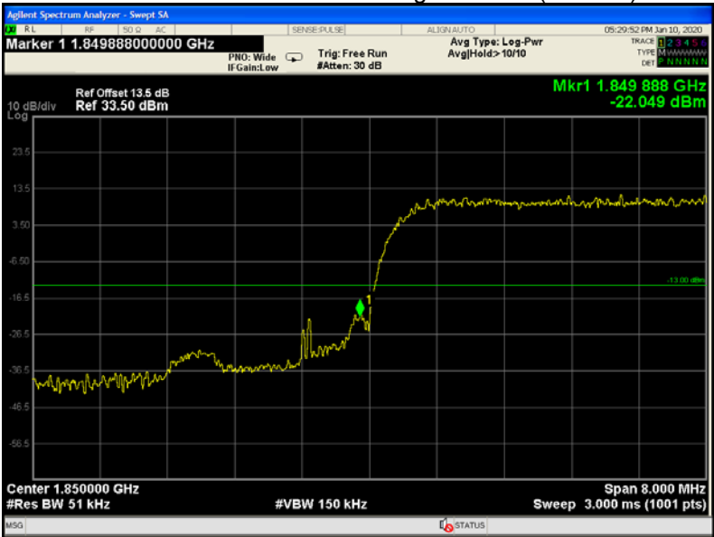
WCDMA band II band edge-left side (HSDPA)
