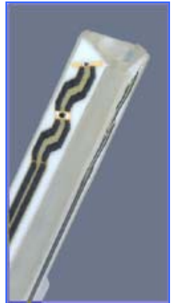
Figure 5. ET3DV6 E-field Probe
