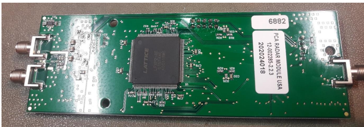
Photo 8: RX board - Bottom view.
