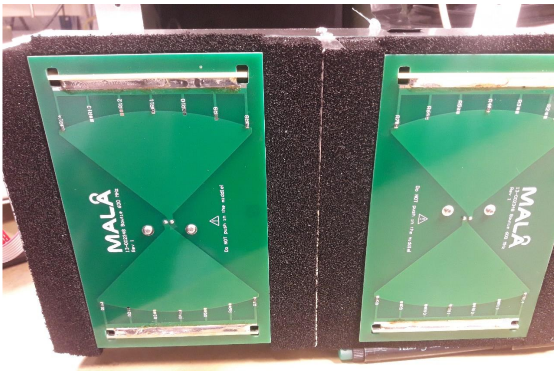
Photo 10: Bottom view of inner shielding box, showing bottom of TX-antenna (left) and RX-antenna (right).
