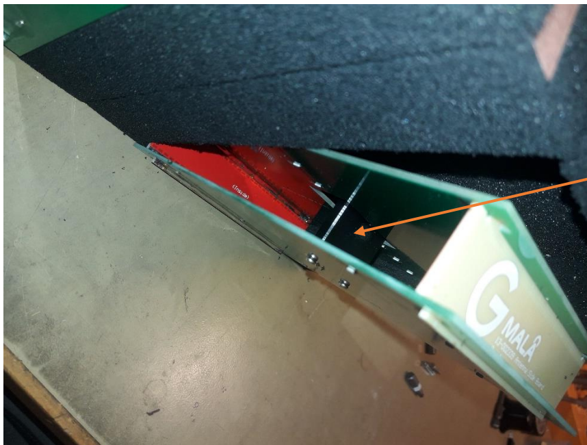
Photo 11: RX-antenna partly pulled out, showing antenna backplane and connection support in centre.
