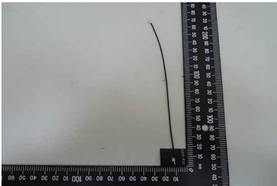
WLAN Antenna – 1 (PIFA Antenna, Model No.: RFA-02-P33-70B-150)
