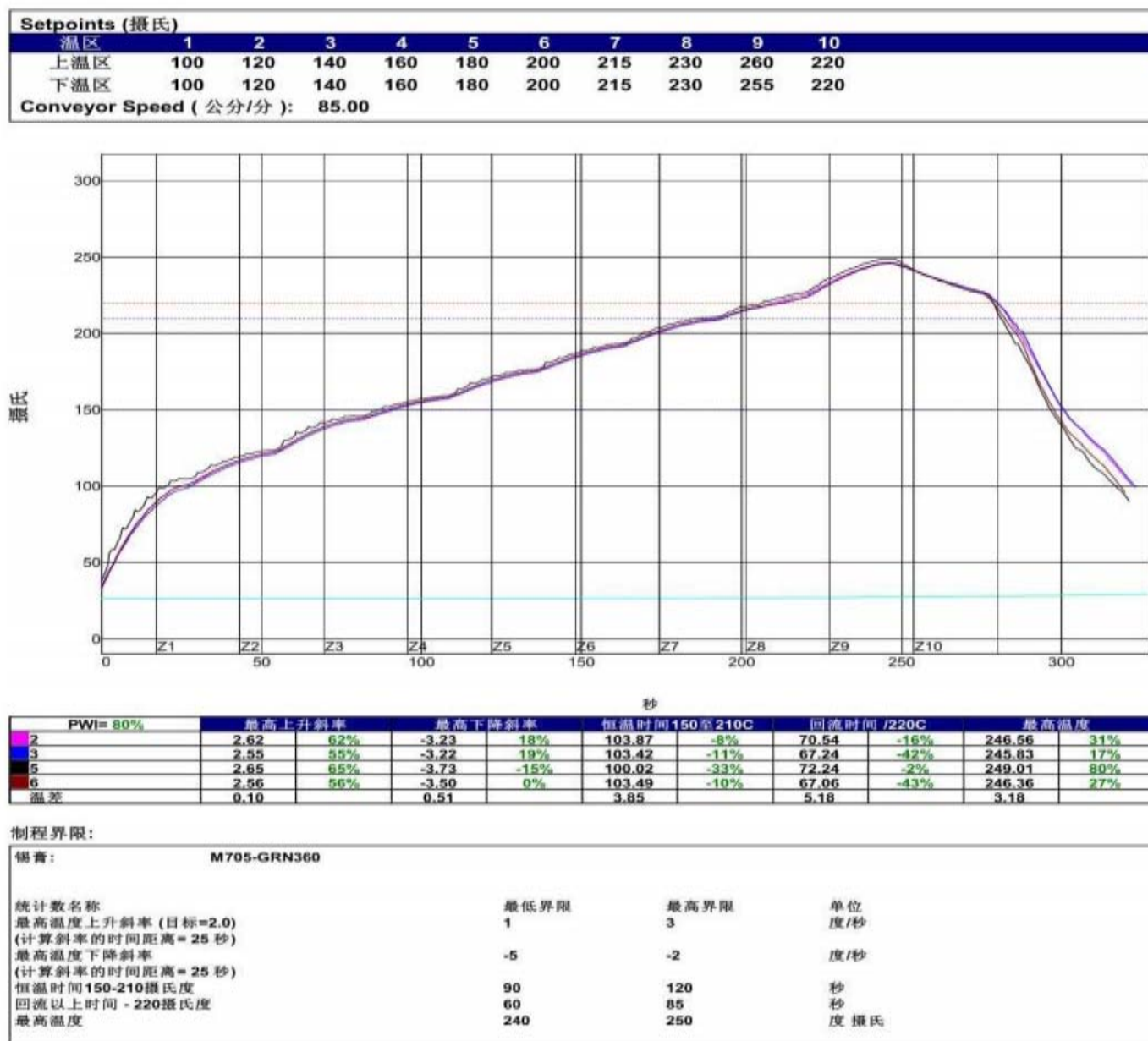
Figure 34 Reflow soldering temperature profile
