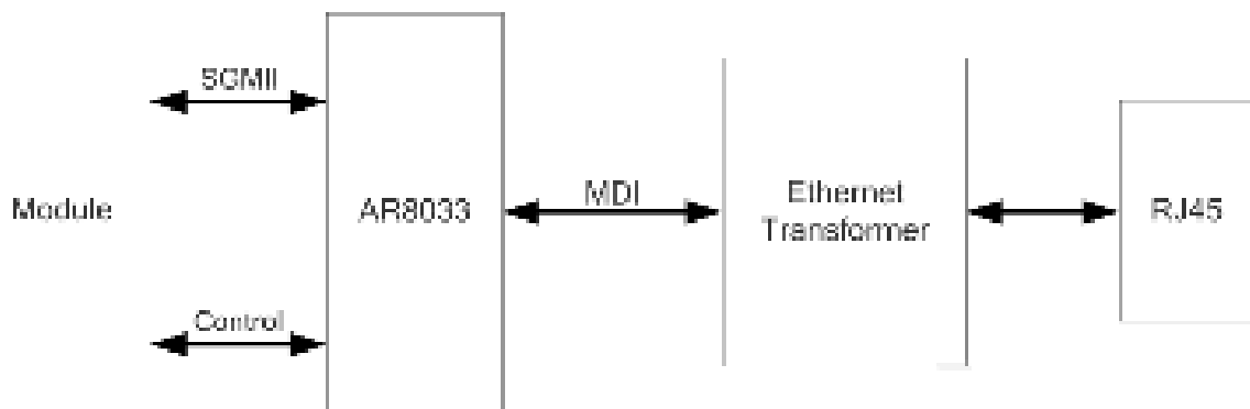
Figure 22 Simplified Block Diagram for Ethernet Application
