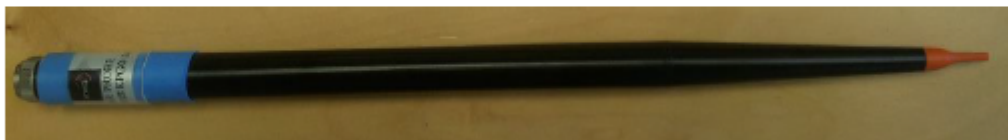
Figure 1 – MVG COMOSAR Dosimetric E field Dipole
