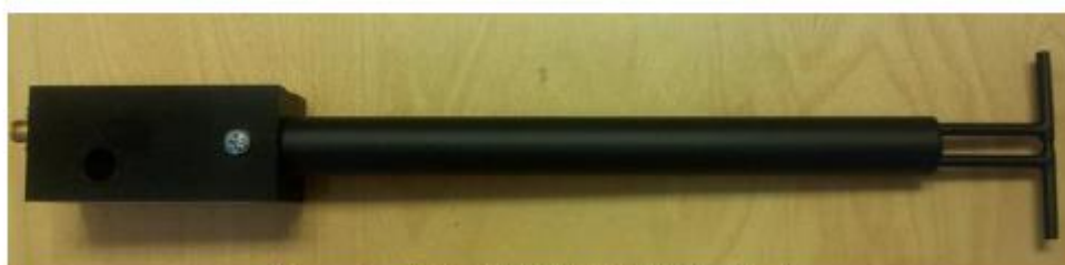
Figure 1 – MVG COMOSAR Validation Dipole
