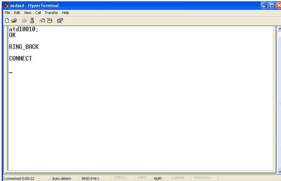
Picture 31: Using HyperTerminal dial number D. The AT Command for Hang up is "AT+CHUP".
