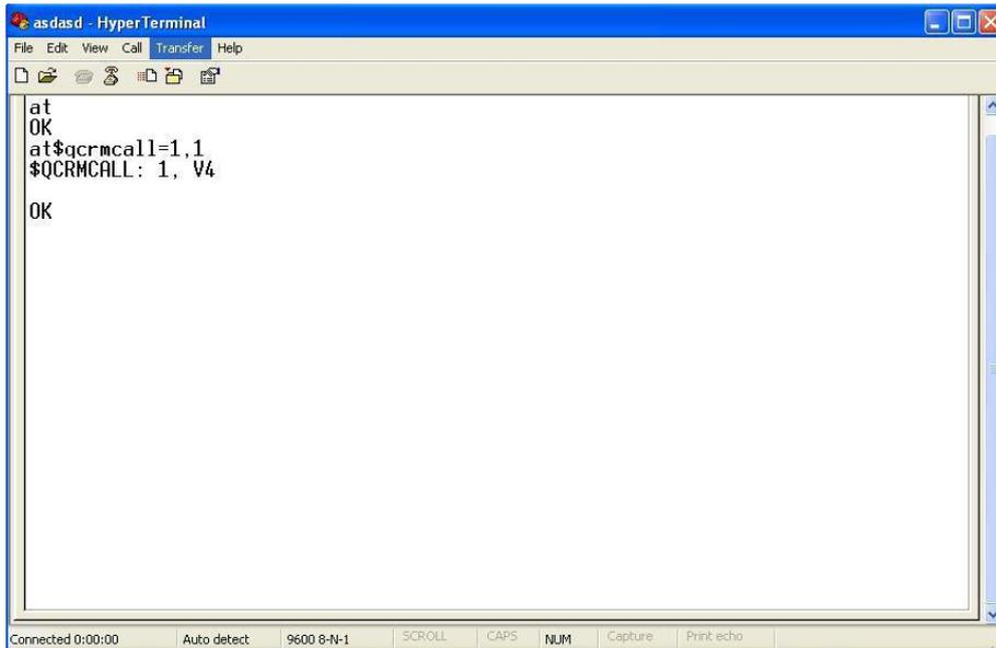
Picture 25: using HyperTerminal to send AT command to NDIS dial
