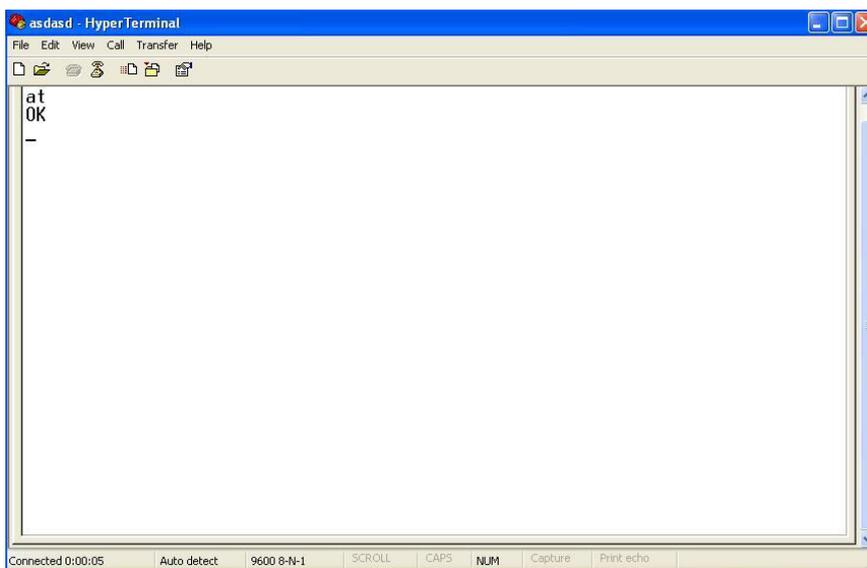
Picture 24: UsingHyperTerminal sending at
