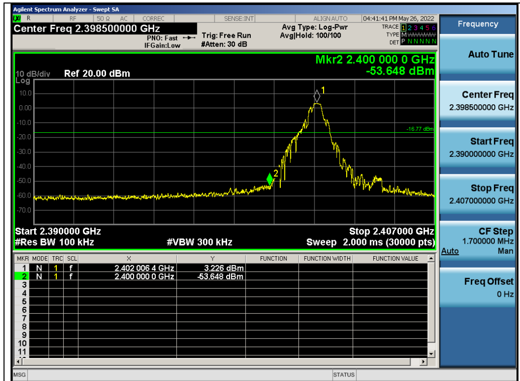
Test_Graph_BR_ANT1_2402_1Mbps_Lower Band Edge Emissions
