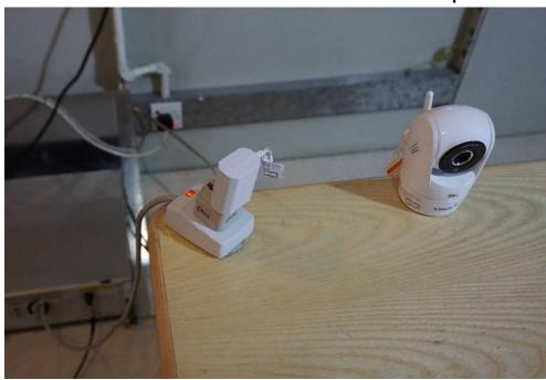
Radiated Emissions (30MHz-1GHz) Test Setup
