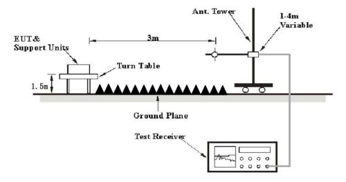
The radiated emission tests were performed in the 3 meters, using the setup accordance with the ANSI C63.10-2013. The specification used was the FCC 15.209, FCC 15.247 limits and RSS-247/RSS-Gen limits.
