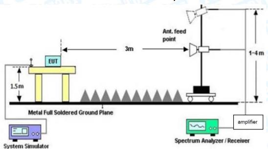
**Above 1GHz Test Setup**
