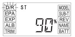
Dual Rate is a percentage of End Point Adjustment. For example, if you set the Steering Dual Rate percentage value to 100%, the steering will travel the same amount as defined by your Steering End Point Adjustment programming. If you set the Steering Dual Rate percentage value to 50%, the steering will travel half that amount.
