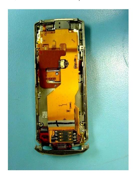
Exhibit 4: INTERNAL VIEW of Vertu FCCID: P7QRHV-5 showing reverse of display module and interconnections.
