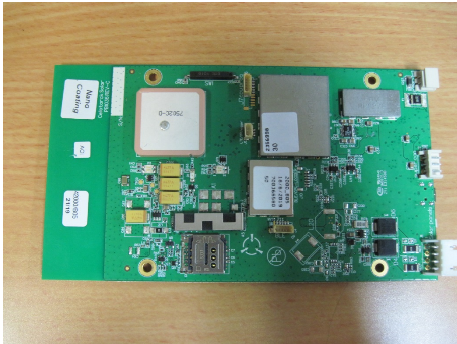
Front of card with the shields removed
