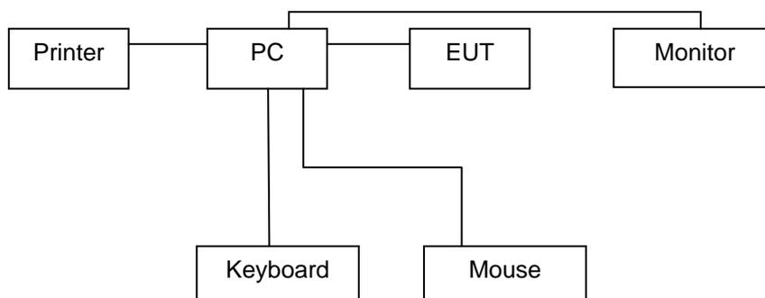
**3.5. Support unit used in test configuration**
