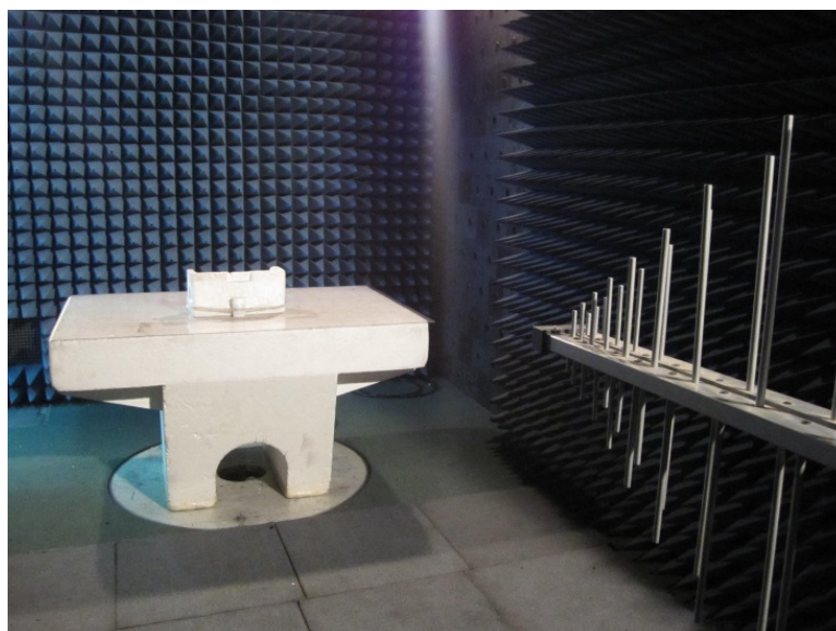
Photograph 8.1.1 Setup for radiated emission measurements in 30-1000 MHz
