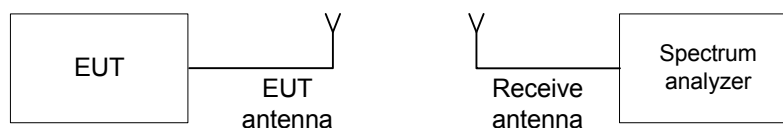
Figure 7.8.1 Band edge emission test setup
