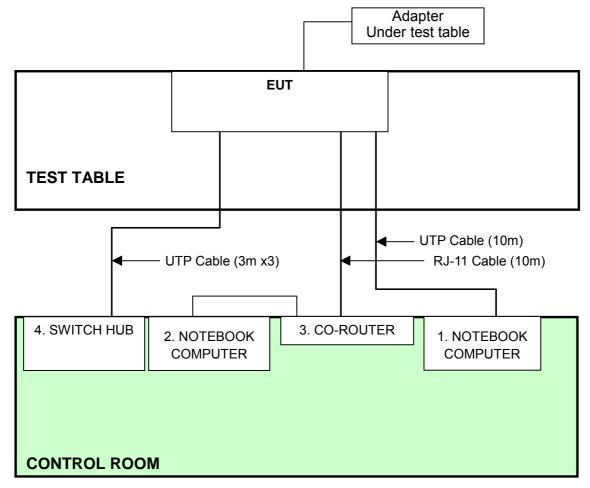
**NOTE:** 1. Support unit 1~4 were kept in the control room during the test.
