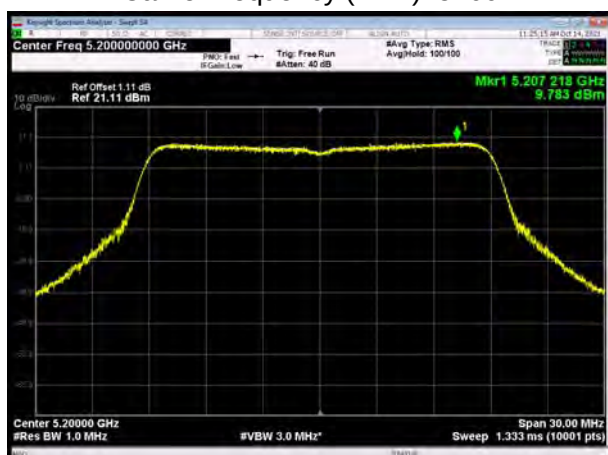
U-NII-1, 802.11ac VHT20 Carrier frequency (MHz): 5240
