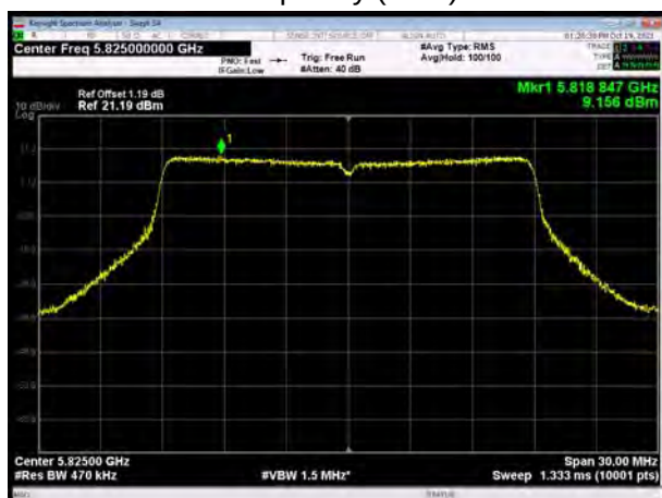
U-NII-3, 802.11ac VHT80 Carrier frequency (MHz): 5775
