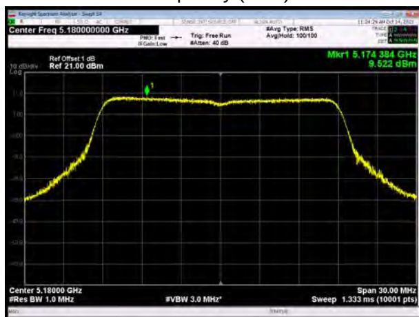
U-NII-1, 802.11ac VHT20 Carrier frequency (MHz): 5200
