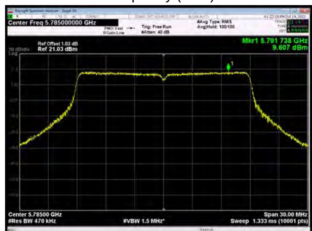
U-NII-3, 802.11ac VHT20 Carrier frequency (MHz): 5785
