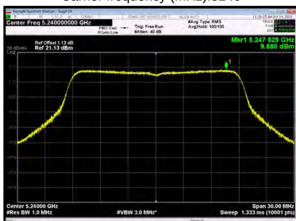
U-NII-1, 802.11ac VHT20 Carrier frequency (MHz): 5240
