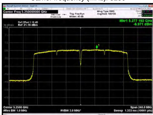
U-NII-2A, 802.11ac VHT160 Carrier frequency (MHz): 5250
