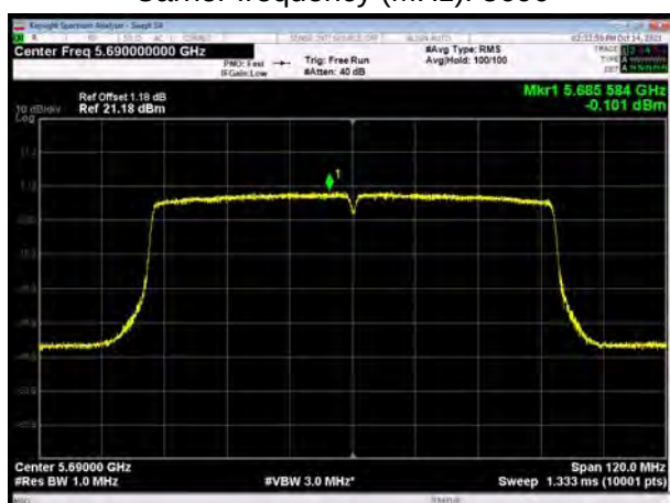
U-NII-2C, 802.11ac VHT80 Carrier frequency (MHz): 5690
