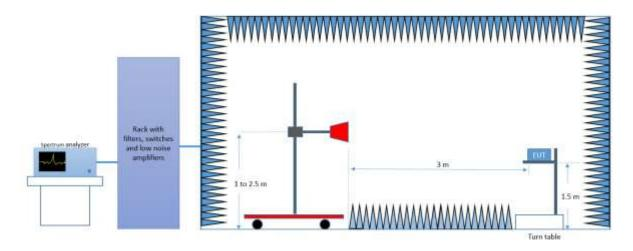
Radiated Setup 18 GHz - 26.5 GHz
