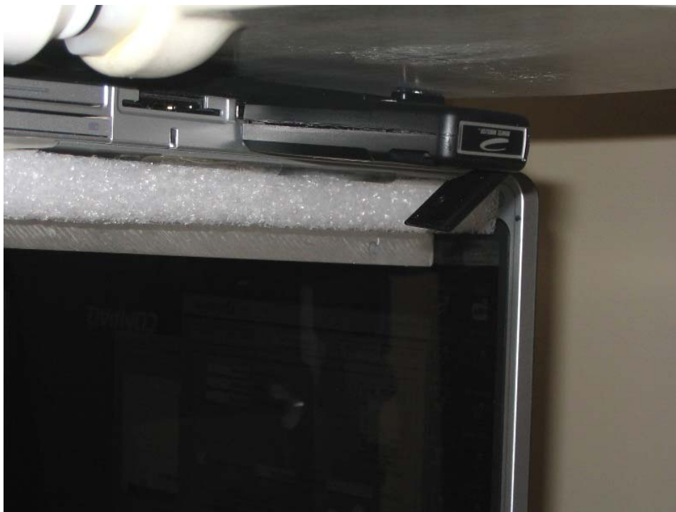
Figure 15: MCD3000 – Compaq Laptop with Antenna at 45 Degrees
