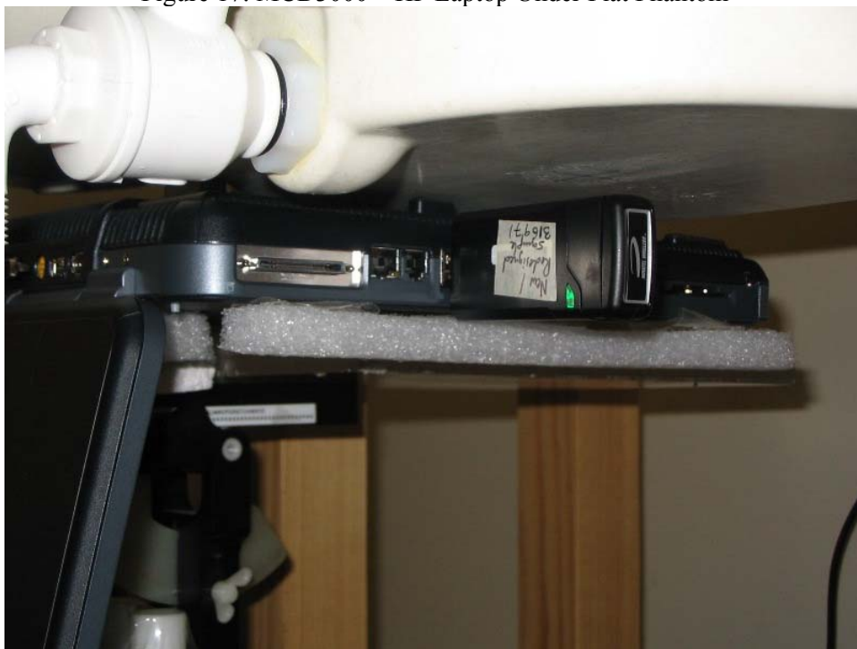
Figure 18: MCD3000 – HP Laptop with Antenna at 0 Degrees
