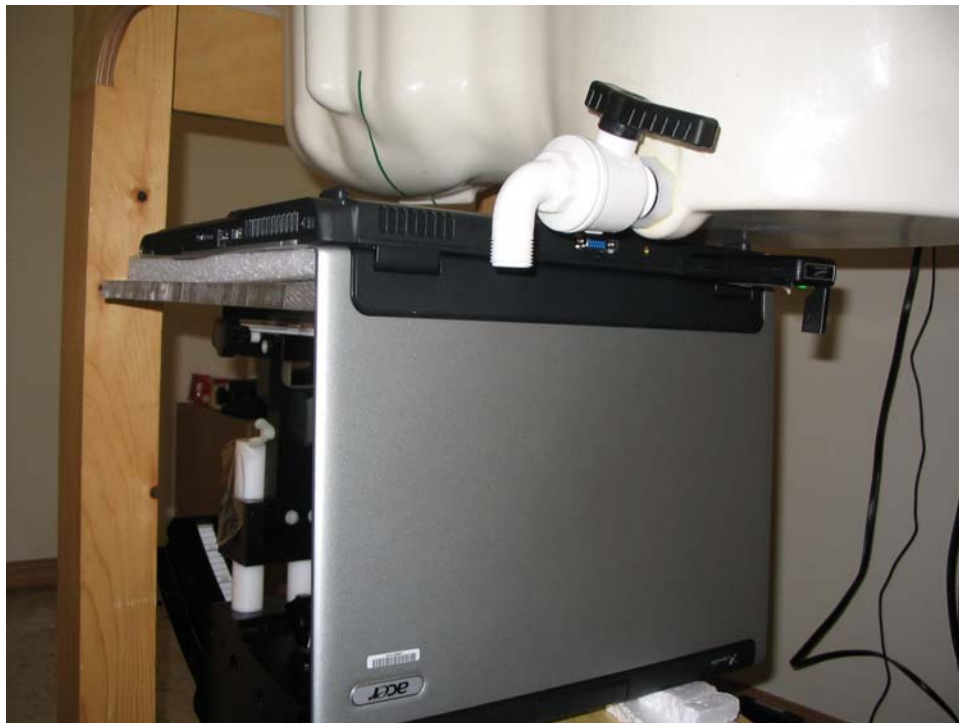
Figure 9: MCD3000 – Acer Laptop Under Flat Phantom
