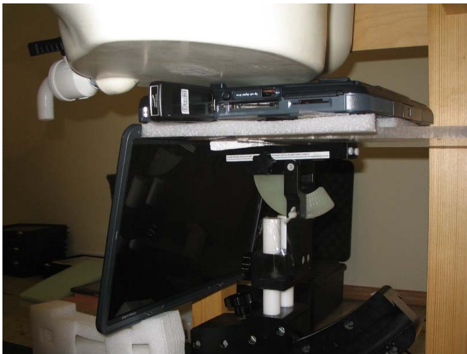
Figure 17: MCD3000 – HP Laptop Under Flat Phantom
