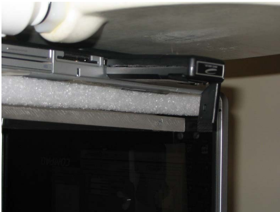
Figure 16: MCD3000 – Compaq Laptop with Antenna at 90 Degrees
