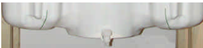
Figure 7.2 SAM Twin Phantom shell
