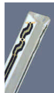
Figure 3.2 Probe Thick-Film Technique
