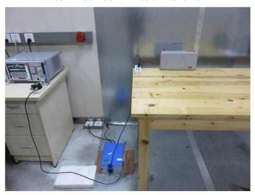
FCC RADIATED EMISSION TEST SETUP
