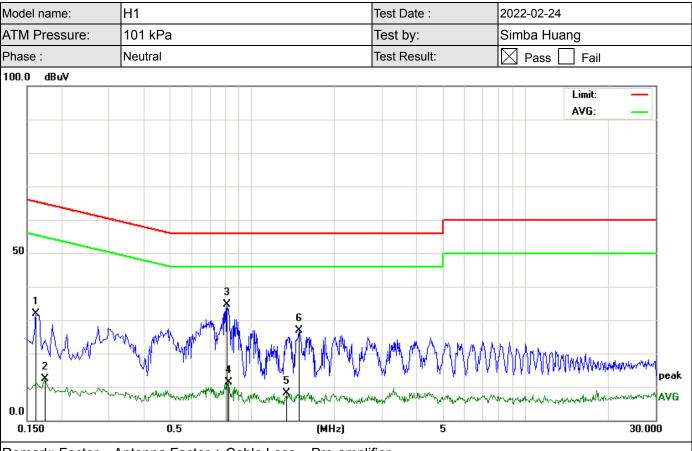
Remark: Factor = Antenna Factor + Cable Loss – Pre-amplifier. Measurement Result=Reading Level +Correct Factor;
