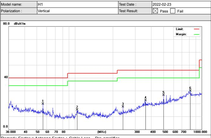
Remark: Factor = Antenna Factor + Cable Loss – Pre-amplifier. Measurement Result=Reading Level +Correct Factor; Over Limit= Measurement Result- Limit;
