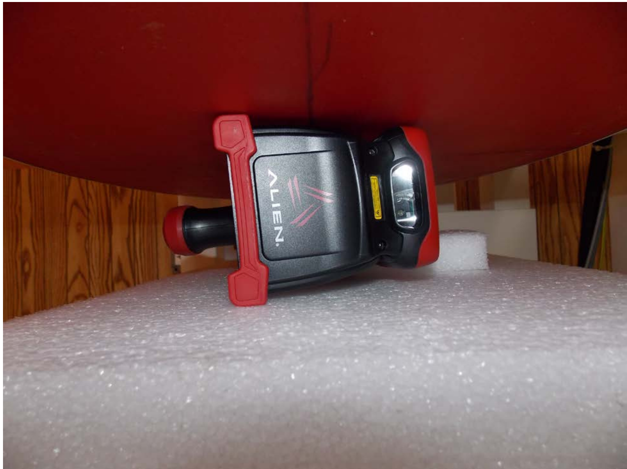
Test Position Side D RFID Testing 0 mm Gap
