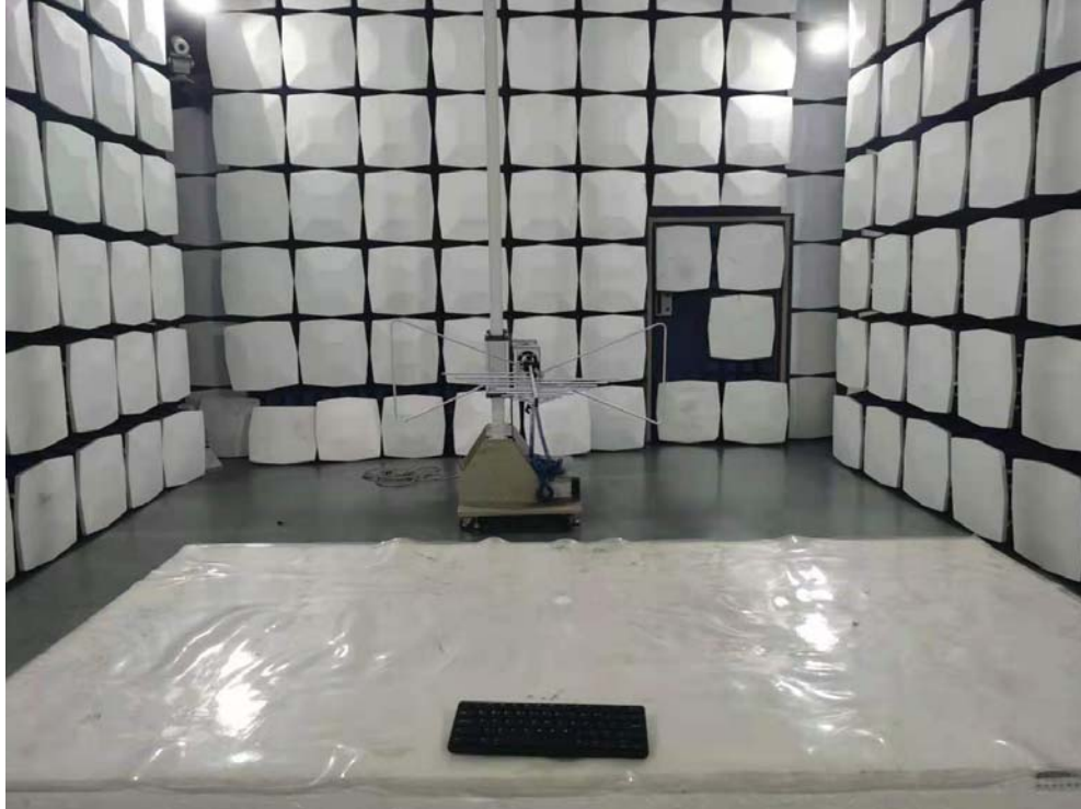
Radiated Emission Test Setup:
