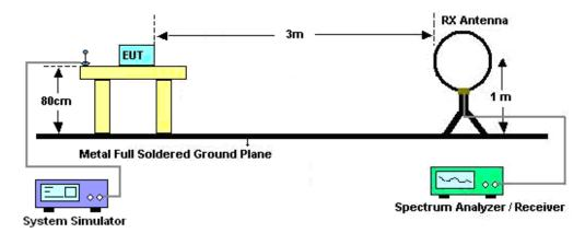
For radiated emissions from 30MHz to 1GHz
