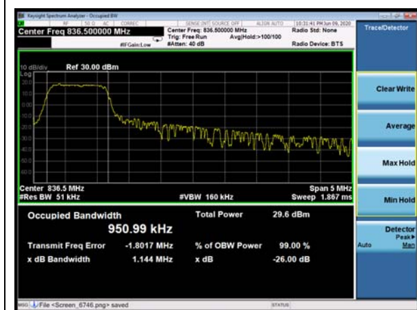
LTE Band 5 16QAM 5MHz CH-Middle
