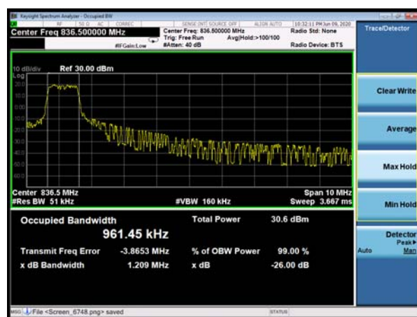
LTE Band 5 16QAM 10MHz CH-Middle
