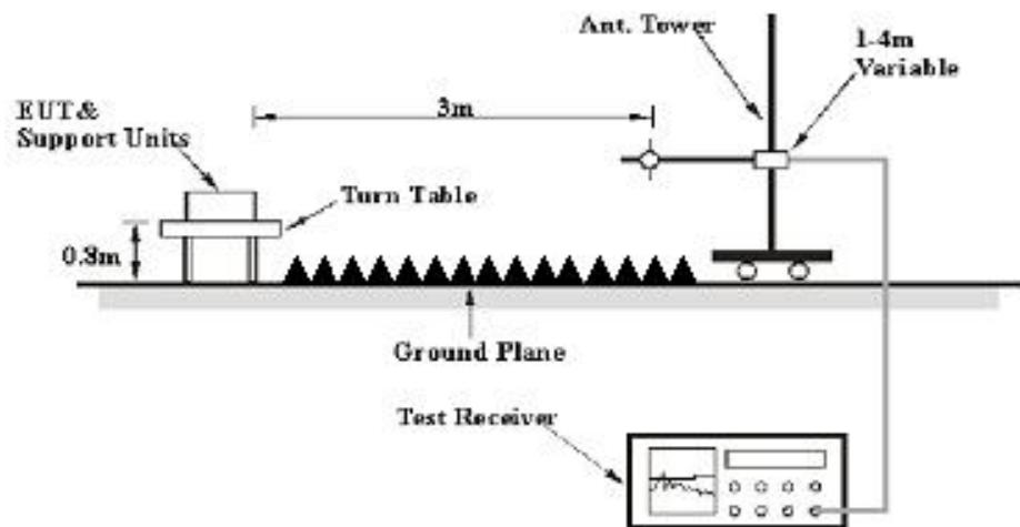
The radiated emission tests were performed at the 3 meters distance, above 1GHz were performed at the 3 meters, using the setup accordance with the ANSI C63.4-2014. The specification used was the FCC Part 15.109 Class B limits.
