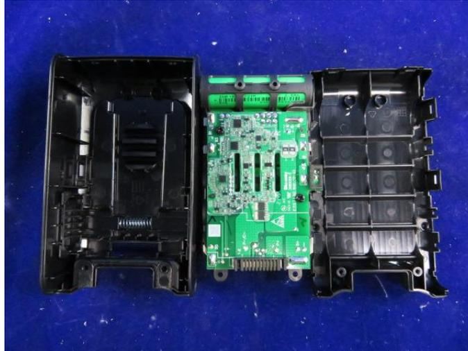
internal view of battery pack VS15-01
