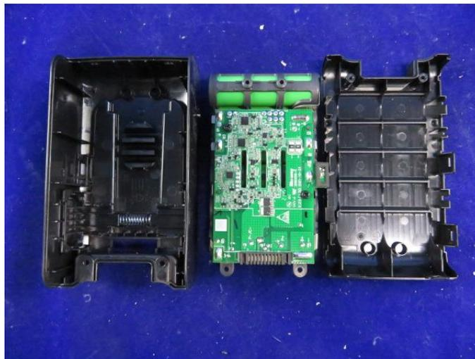
internal view of battery pack VS15-02
