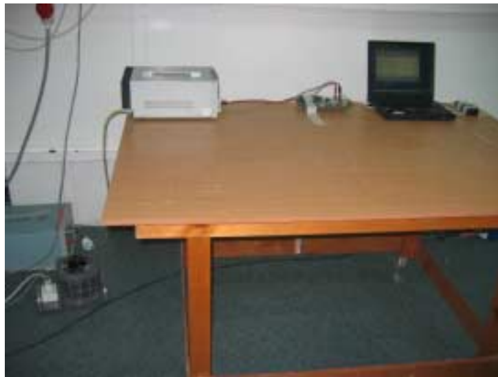
Photograph 7.1.1 Setup for conducted emission measurements
