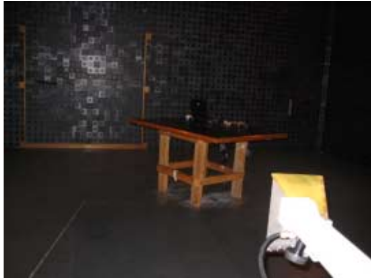
Photograph 7.2.2 Setup for radiated emission measurements, EUT cabling
