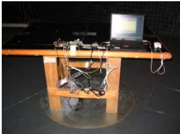
Photograph 7.2.2 Setup for radiated emission measurements, EUT cabling
