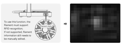
Align the chip on the filament with the RFID recognition area on the machine to scan and automatically read the filament information;
