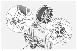
**4** A. Press down on the wrench; B. Remove the filament;
