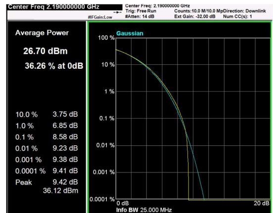
Channel: MIDDLE, Modulation: 64QAM, BW=20MHz, CCDF
