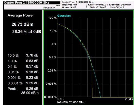
Channel: BOTTOM, Modulation: 64QAM, BW=10MHz, CCDF
