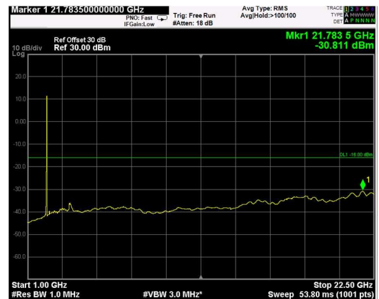
Channel: MIDDLE, Modulation: QPSK, BW=5MHz, Range: Upper
