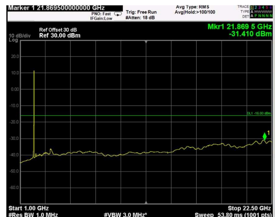
Channel: TOP, Modulation: 64QAM, BW=5MHz, Range: Upper
