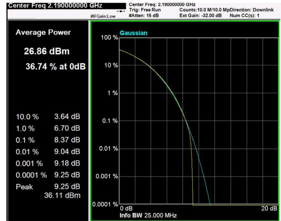
Channel: MIDDLE, Modulation: 256QAM, BW=20MHz, CCDF
