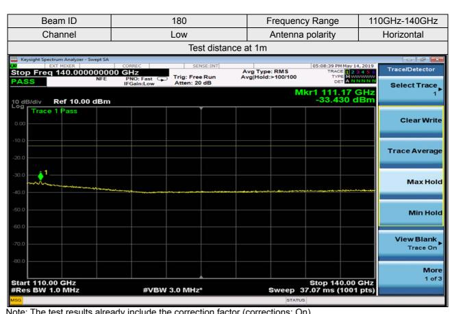
Note: The test results already include the correction factor (corrections: On).
