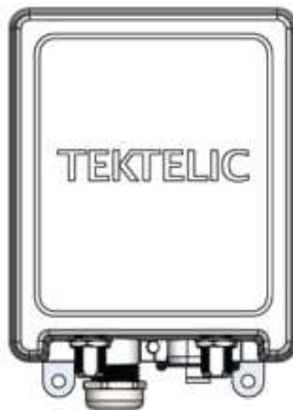
Figure 6: Kona Enterprise Gateway Module Wall Mounting Orientation
