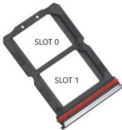
Figure 4: SIM Tray Layout of Slot 0 and Slot 1
