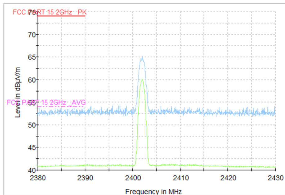
Fig. 55 Radiated Band Edges (8DPSK, Ch0, 2380GHz ~ 2450GHz)
