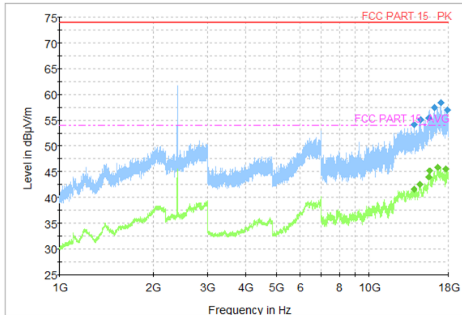
Fig. 52 Radiated Spurious Emission (8DPSK, Ch0, 1GHz ~ 18GHz)
