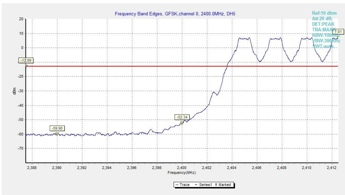
Fig. 1 Band Edges (GFSK, Ch 0, Hopping ON)
