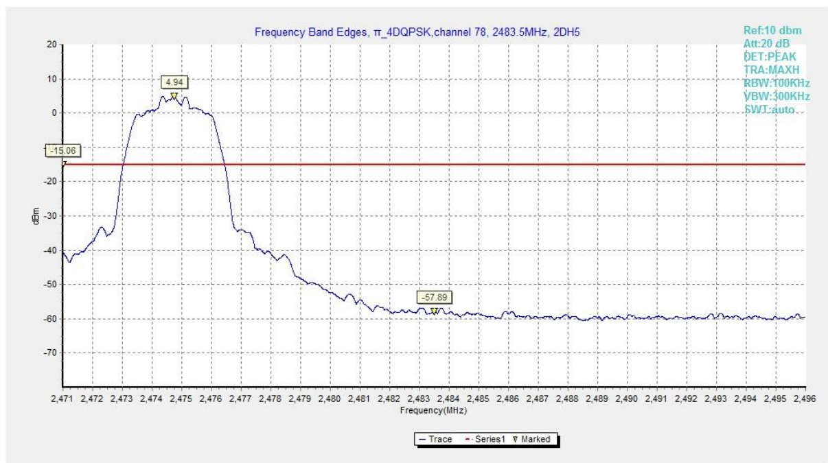
Fig. 10 Band Edges ( \pi/4 DQPSK, Ch 78, Hopping OFF)
