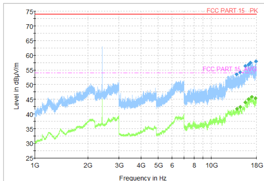
Fig. 47 Radiated Spurious Emission ( \pi/4 DQPSK, Ch0, 1GHz ~ 18GHz)
