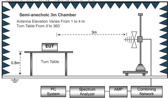
(C) Radiated Emission Test-Up Frequency Above 1GHz
